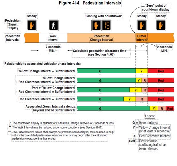
Countdown pedestrian signals, which are required by the MUTCD when the pedestrian change interval is longer than 7 seconds, display the number of seconds remaining until the termination of the pedestrian change interval.
