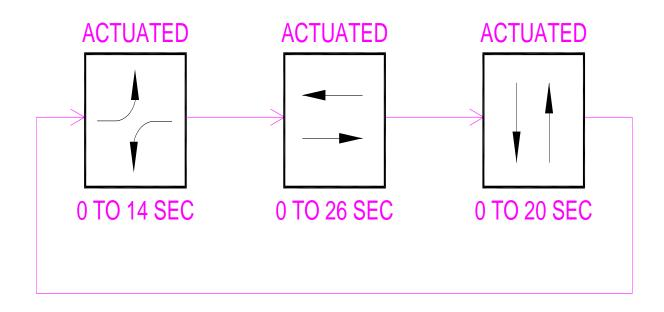
The cycle length will vary from cycle to cycle with a maximum cycle length for this example of 60 seconds. Fully-actuated controllers offer the most sophisticated timing features and capabilities so the remaining discussion centers on these types of controllers.
